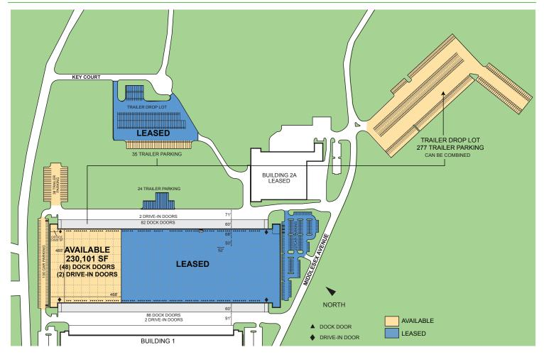
WAREHOUSE: 226,281 SF OFFICE: 3,820 SF TOTAL FLOOR PRINT: 230,101 SF CLEAR HEIGHT: 36' DOCK DOORS: 48 DRIVE-IN DOORS: COLUMN SPACING: 52' x 50' CAR PARKING: 130 STALLS TRAILER PARKING: 73 STALLS ADDITIONAL TRAILER PARKING: UP TO 526 STALLS (277 STALLS IN DROP LOT & 249 STALLS IN LOT "D" NOT PICTURED)
